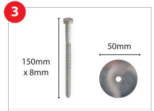
150 x 8mm concrete galvanized bolts are used to fix the expanded metal to the wall. These fixings go right through in to the wall structure. Insert fixings at a slight upwards angle.
