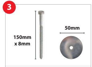
150 x 8mm concrete galvanized bolts are used to fix the expanded metal to the wall. These fixings go right through in to the wall structure. Insert fixings at a slight upwards angle.
